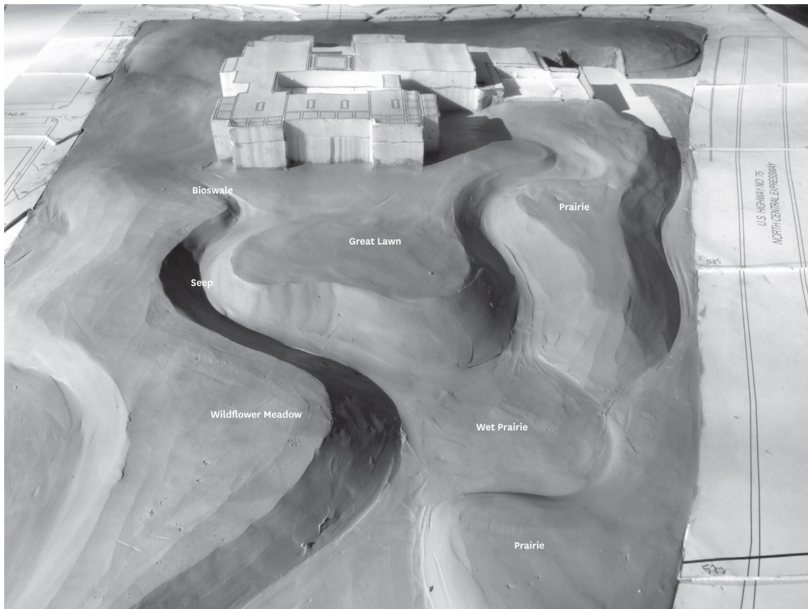
FIGURE 6. The building excavation created 100,000 cubic yards of excess fill that needed to be used on site. Clay study models like this showed possibilities for configuring topography.
