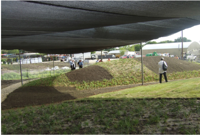
FIGURE 5. A mounded mock-up was used to monitor seed mixes, slope stability, soil type, and water needs over 15 months. Test plots for native and commercial lawns were also observed.
