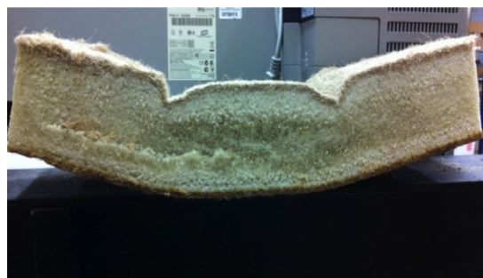
FIGURE 4.5. Deformed Tung-treated hemp panel.
