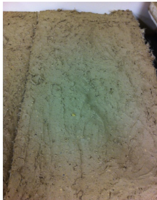
FIGURE 3.2. Earth plaster treated hemp fibre specimens.
