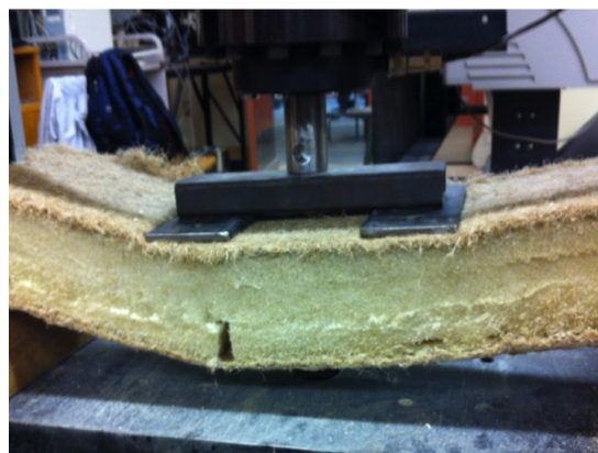
FIGURE 4.4. Flexural earth plaster hemp specimen.
