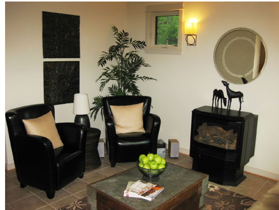
The Mantis—a high efficiency gas furnace disguised as a free-standing fireplace.
