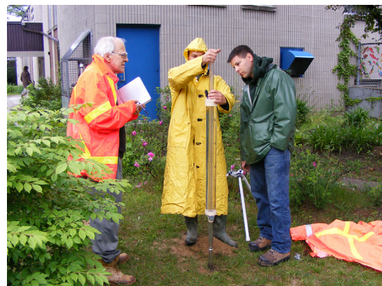
FIGURE 17. In-situ infiltration testing using the Guelph Permeameter Apparatus and Testing Methods.
