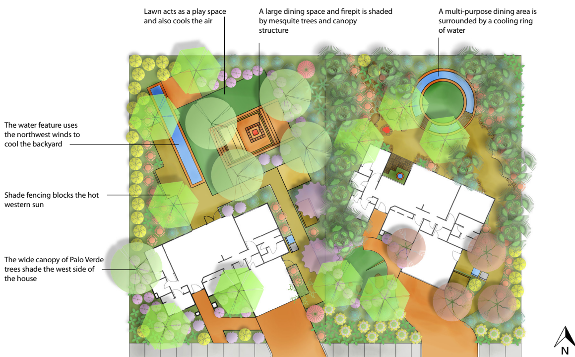
FIGURE 7. Passive design techniques applied in Palm Desert. Design by Stephen Nunez.
