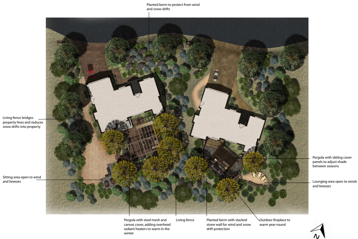
FIGURE 9. Passive design techniques applied in Truckee. Design by Richard Kane.
