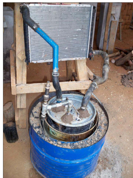
FIGURE 8. Completed biodiesel processor built at the ACREST facility in Cameroon.
