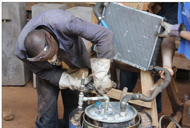
FIGURE 7. A technician assembles the low cost biodiesel reactor at the ACREST facility in Cameroon.
