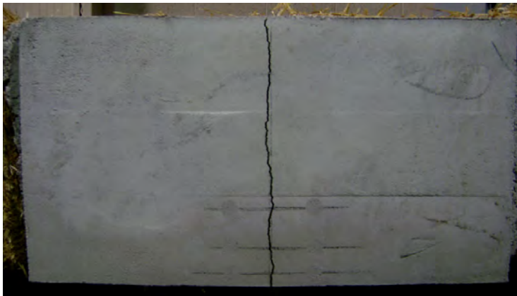
FIGURE 12. Plastered straw bale panel, failed by vertical tensile cracking.
