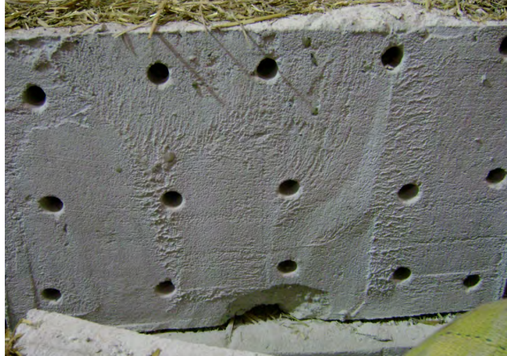
FIGURE 10. Holes drilled in the plaster skin after the completion of each test to permit measurements of the plaster thickness.
