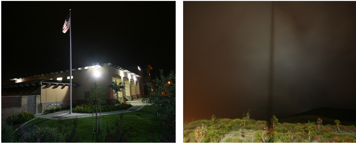
FIGURE 6. A LEED Gold certified fire station in San Marcos, CA, where dark-sky friendly outdoor lighting was not taken into consideration. The station's flag lighting is a major source of glare. The light is bright enough that when low clouds blow in from the nearby Pacific Ocean, one can easily see the shadow of the flag in the sky.
