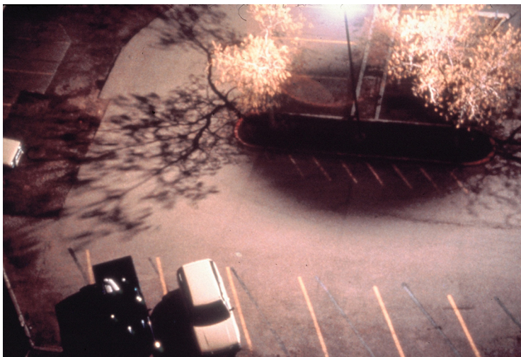
FIGURE 3. An example of the poor lighting environment created by an unshielded post-top lamp. In this case, harsh shadows exist directly under the light source. (credit: IDA)
