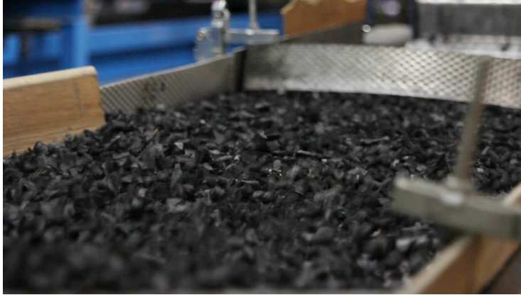
Processing of recycled tire crumb rubber by RTR, Winnipeg, Manitoba, Canada.
