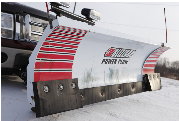
Rubber edge fabricated from mining tires installed on metal snow plow blade.
