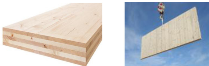
FIGURE 1. Prefabricated cross-laminated panels are engineered load-bearing jumbo panels, consisting of a series of layers, bonded together timber boards (usually spruce, larch or pine) with structural adhesives, forming a solid timber panel with each layer of the panel alternating between longitudinal and transverse lamellae. CLT panels can be up to format 3.2 × 16 metres (approx. 10 × 45 feet) in size.
