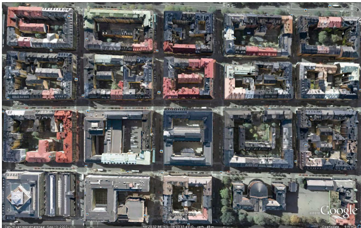
FIGURE 9. Less natural elements in European urban courtyards in cold regions; Stockholm, Sweden. The courtyards are designed to obstruct the cold winds (picture from Google Earth).
