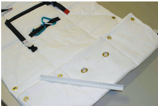
FIGURE 10. CTB Water Wall input ports for forward osmosis treatment and recovery of wastewater.
