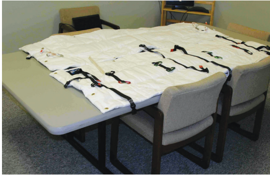
FIGURE 10. CTB Water Wall input ports for forward osmosis treatment and recovery of wastewater.
