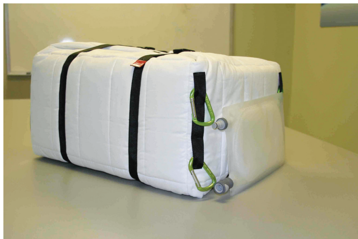
FIGURE 8. Folded CTB Water Wall Architecture Element Demonstrator with the current space flight-rated FO bag alongside for scale.
