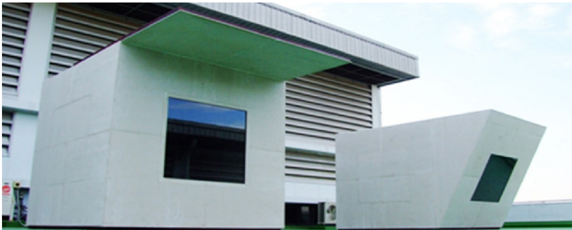
FIGURE 3. Test cells of shading system (left) and tilted façade system (right).
