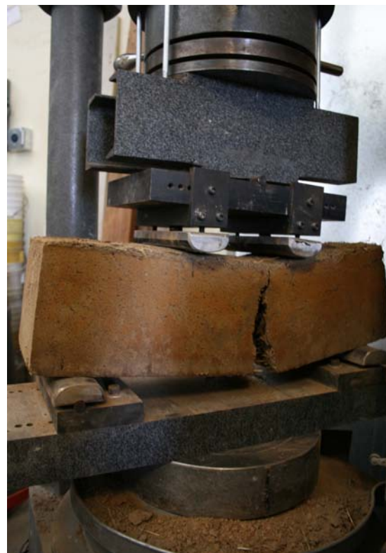
FIGURE 4. Modulus of rupture test setup.
