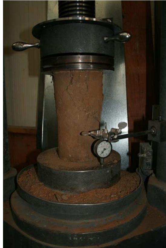
FIGURE 5. Modulus of elasticity test setup.
