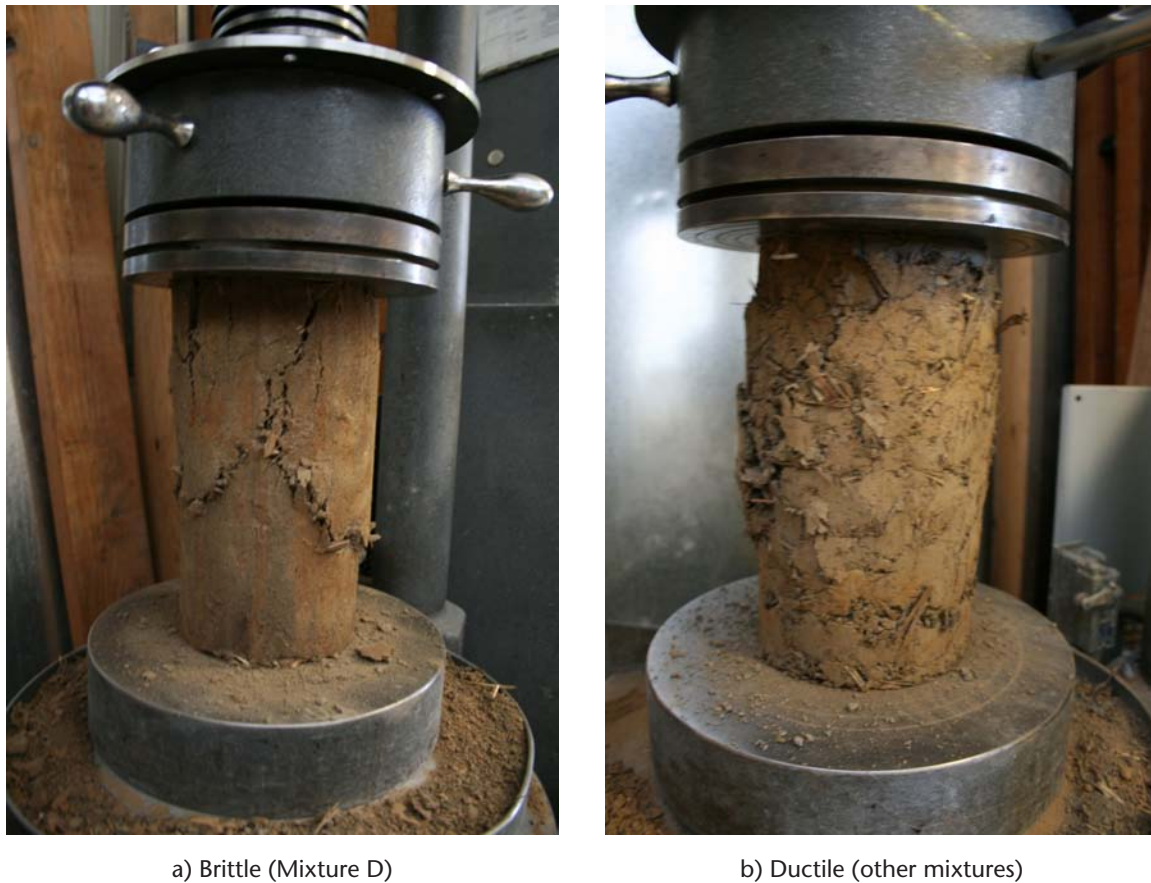
FIGURE 9. Failure modes during unconfined compression tests.
