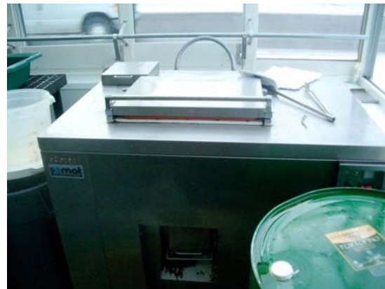
FIGURE 12. High Speed Aerobic Compostable Waste Dehydrator.
