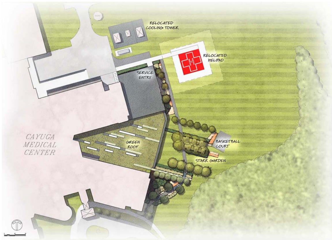
FIGURE 6. The site plan for the green roof at the Laboratory Addition maximizes views from inside the hospital and continues the green roof geometry on the ground plane in gardens and seating areas.
