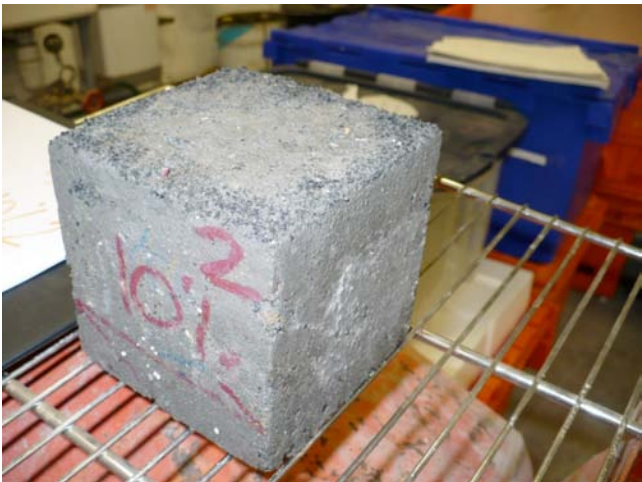
PLATE 4. 10% Rubber sample at 50 freeze/thaw cycles.
