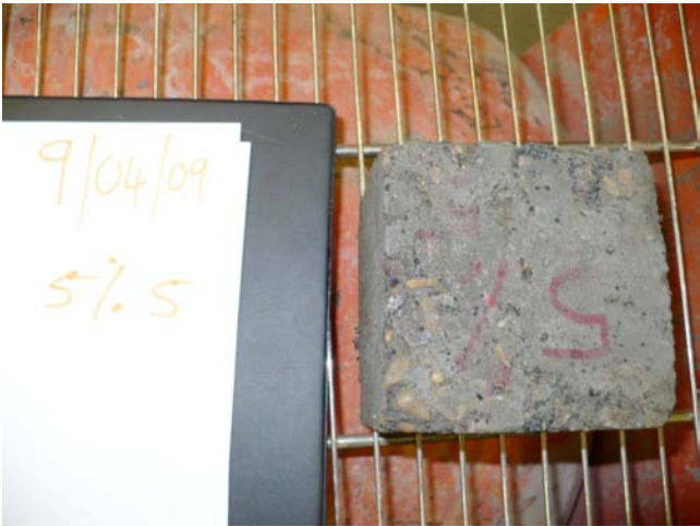
PLATE 3. 0.5% Rubber sample at 50 freeze/thaw cycles.
