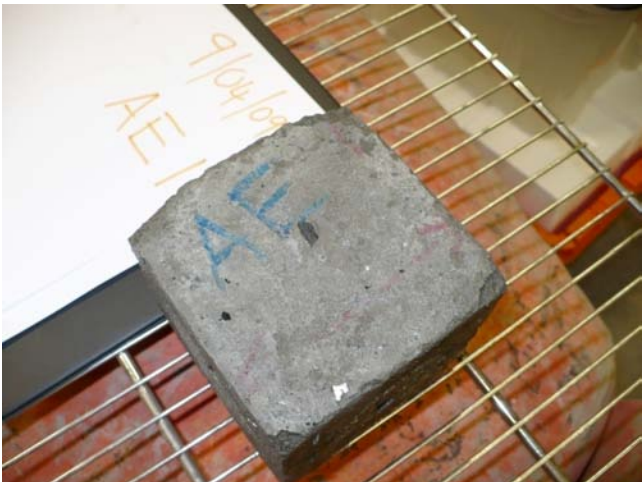
PLATE 2. Air Entrained sample at 50 freeze/thaw cycles.
