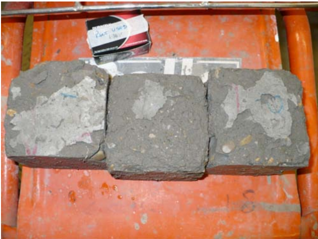
PLATE 1. Plain concrete cubes at 50 freeze/thaw cycles.
