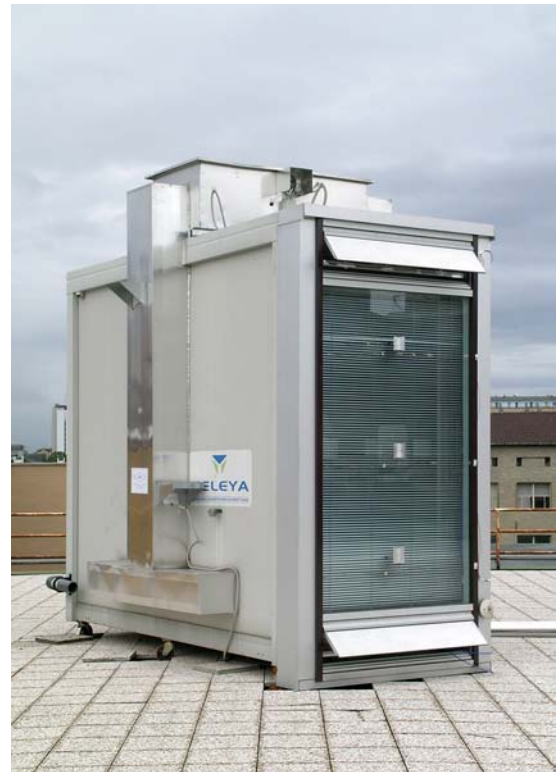
FIGURE 2. The DSF tested at the TWINS facility.
