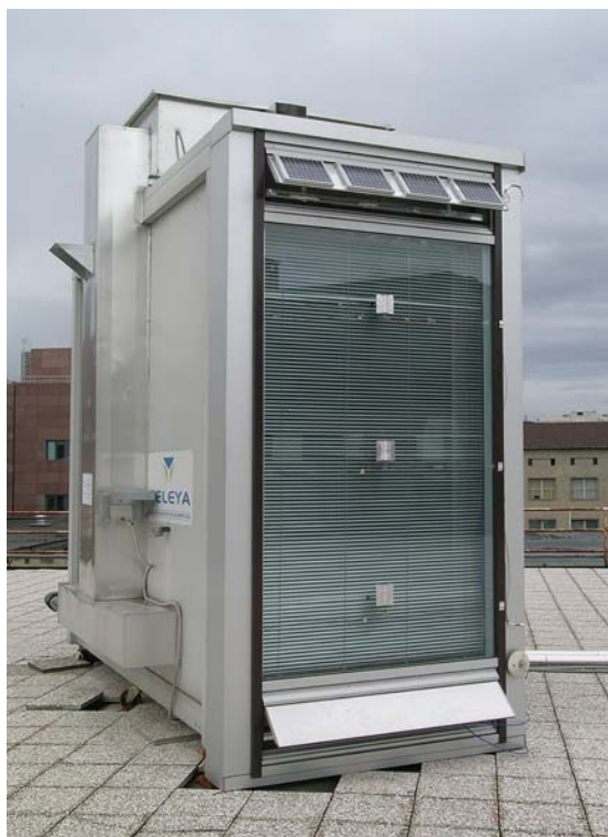
FIGURE 11. The Hybrid Ventilated DSF.
