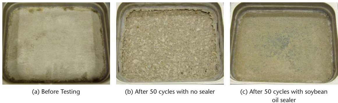
FIGURE 4. 50S-VA Deicer Testing Results.
