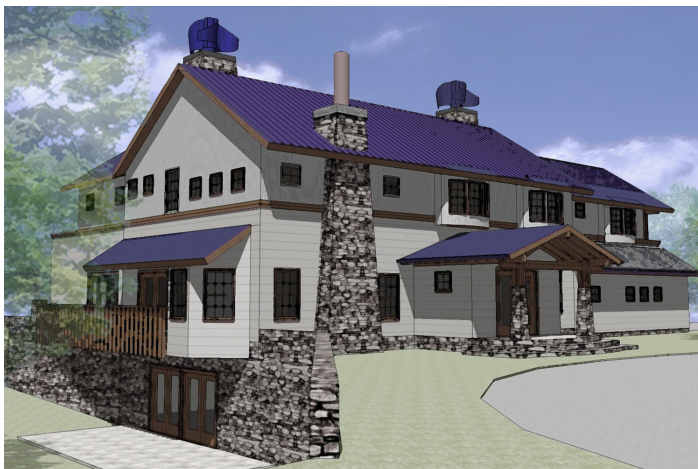
Sketch-Up model showing two 2.4-kW roof-mounted Mag wind units.
