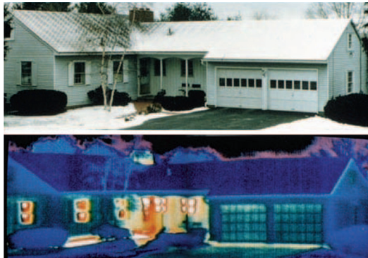
FIGURE 3. An infrared camera measures temperatures thus indicating the best and least insulated parts of the home. Source: U.S. Department of Energy.
