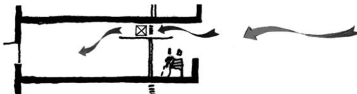
FIGURE 11. Cross section of typical office/tutorial room in air conditioned mode.
