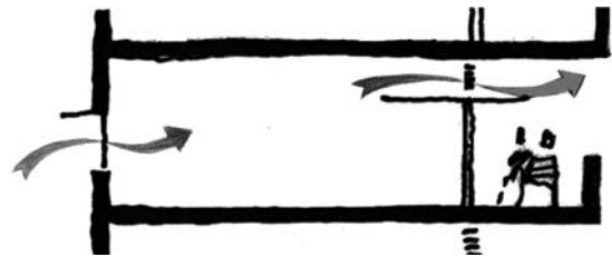
FIGURE 10. Cross section of typical office/tutorial room in natural ventilation mode.
