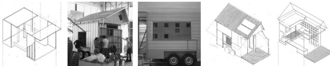
FIGURE 2. (left to right): the 'bookends'; C2, attaching the folding deck; C2, exterior; C2, drawings describing the external and internal arrangements.
