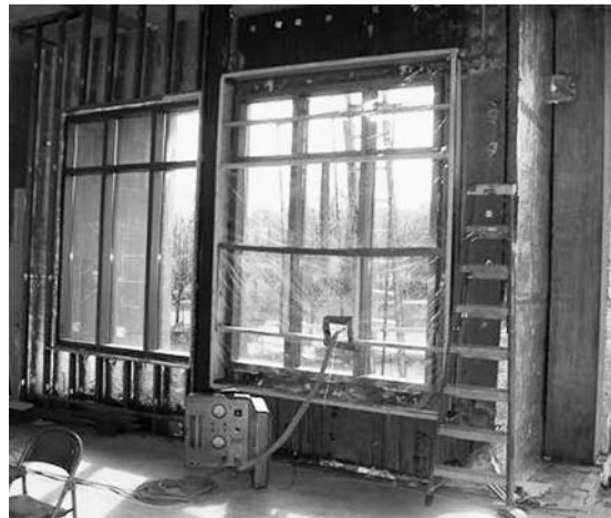
FIGURE 11. This photo shows an aluminum window field test used to verify resistance to water infiltration.
