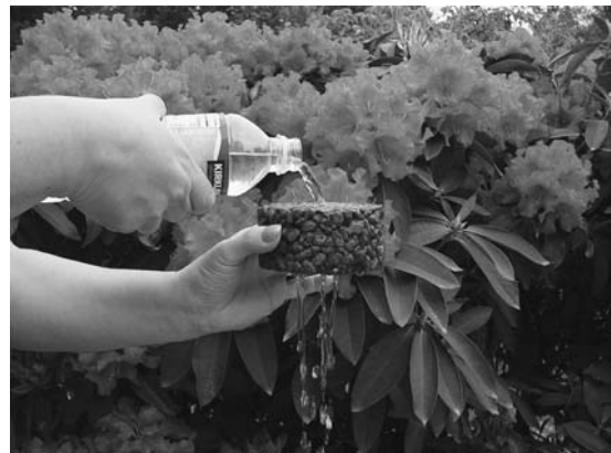
FIGURE 1. Pervious concrete pavements are able to pass flows of water in excess of even the most severe storm rainfall intensities.
