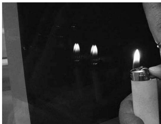
FIGURE 11. Using a light source to check for low-e
