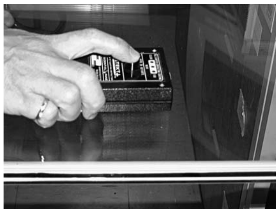
FIGURE 10. Electronic detection of low-e coating
