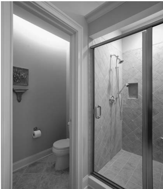
FIGURE 5. For better visibility, a light fixture should be placed in the shower or bath area. Recessed downlights to light the vanity countertop should never be used; lighting from the sides of the mirror is much better for grooming. (Photograph by Michael Kalla.)
