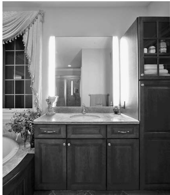
FIGURE 5. For better visibility, a light fixture should be placed in the shower or bath area. Recessed downlights to light the vanity countertop should never be used; lighting from the sides of the mirror is much better for grooming. (Photograph by Michael Kalla.)
