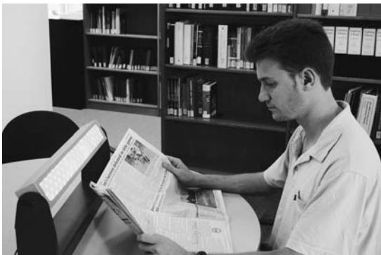
FIGURES 8A AND 8B. Light boxes using blue LEDs peaking at 470 nm and delivering 30 lx at the cornea are a good solution for healthcare applications.
