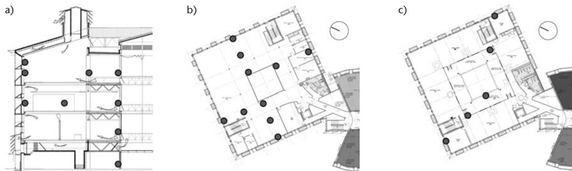
Figure 3. Positions of Hobo dataloggers projected in section (a) and in plan on Levels 3 (b) and 4 (c).
