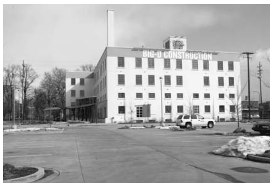
FIGURE 9. Lighter colored concrete was selected for the parking lot since it reduces heat absorption during the day while lighting systems were selected to eliminate light pollution and trespass at night (©2008, Robert A. Young, all rights reserved).
