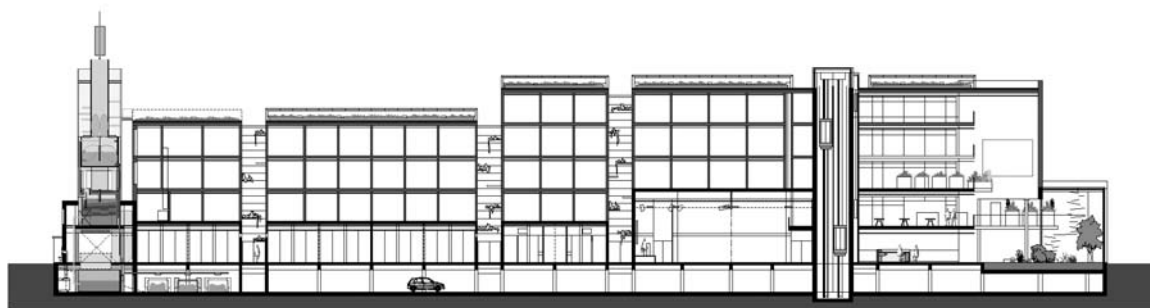
FIGURE 5. Longitudinal section over the EVA Centre with integrated Sustainable Implant (left).
