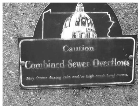
FIGURE 15. A warning sign near a CSO outlet in Harrisburg, Pennsylvania. Combined sewer overflows are among the earliest sewer systems and were designed to carry both stormwater and sewage to a treatment plant. However, in large storms the flow capacity of these systems can be exceeded and the overflow is dumped directly into water bodies. The overflow often contains untreated municipal wastewater, raw sewage, industrial waste, debris, and other pollutants, and it poses a major threat to human health and the environment. (Photo courtesy of Christopher J. Sutton, Western Illinois University.)
