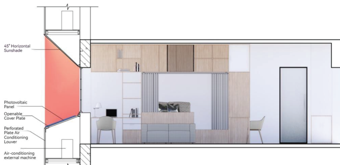
FIGURE 37. Schematic construction of PV sunshade window coverings.
