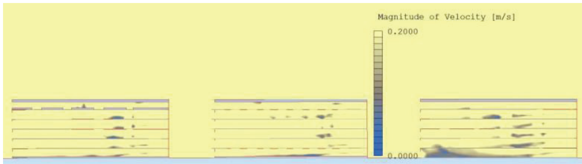
FIGURE 19. Layout 1, Layout 2, and Layout 3 wind environments simulating static wind zone conditions.
