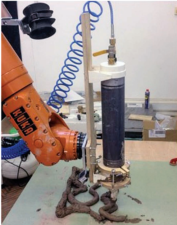
FIGURE 6. Manually controlled compressor used to 3DP cob (Courtesy of Reyes et al. 2018).
