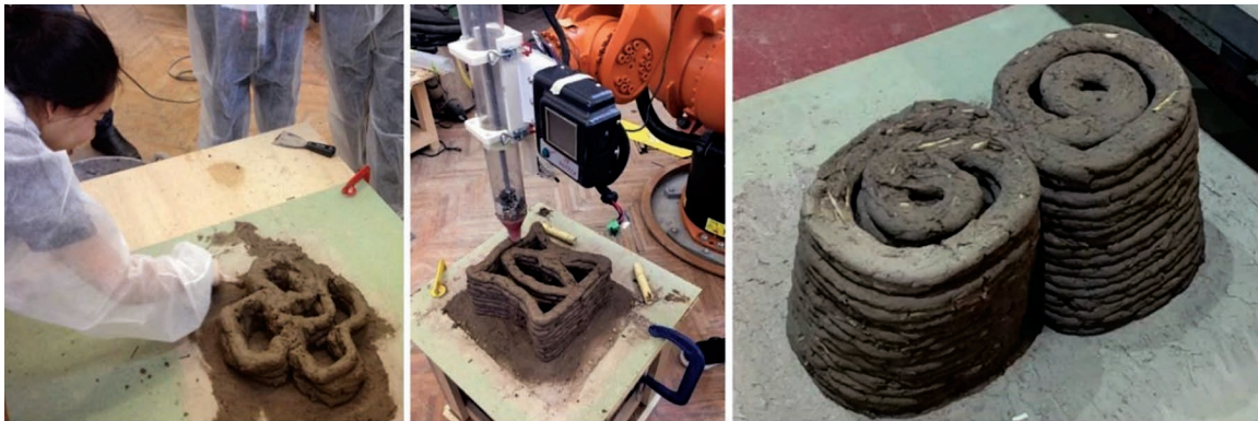
FIGURE 7. The effect of different extrusion systems and different mixtures on the printed cob structure (Courtesy of Reyes et al. 2018).
