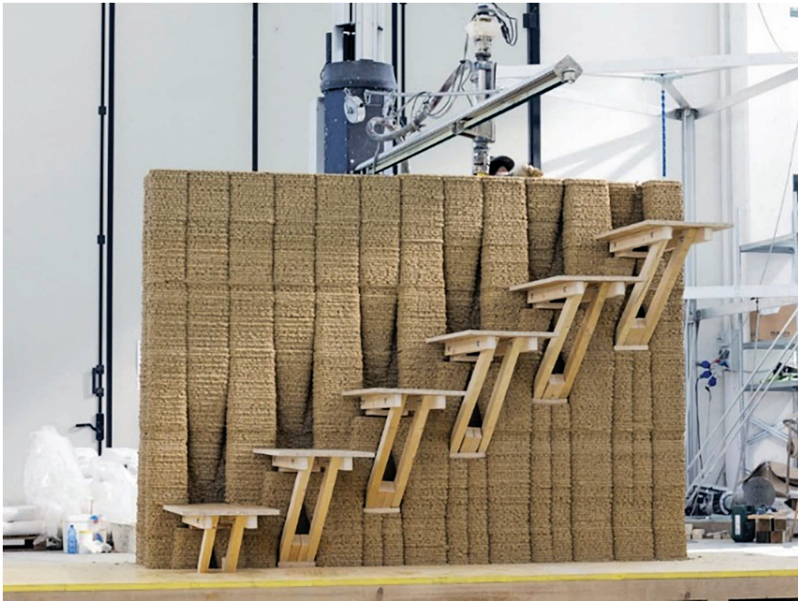
FIGURE 14. 3DP earth-based load bearing wall with embedded stairs (Courtesy of Chiusoli 2019).
