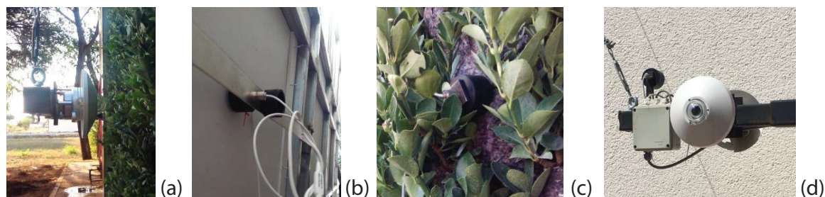
FIGURE 10. Images and location of the sensors: (a) pyranometer in front of VFS, (b) infrared sensors measuring exterior surface temperature of vegetated wall and back side of PVC panel, (c) infrared sensor measuring surface temperature of geotextile felt, and (d) pyranometers in front of RFS
