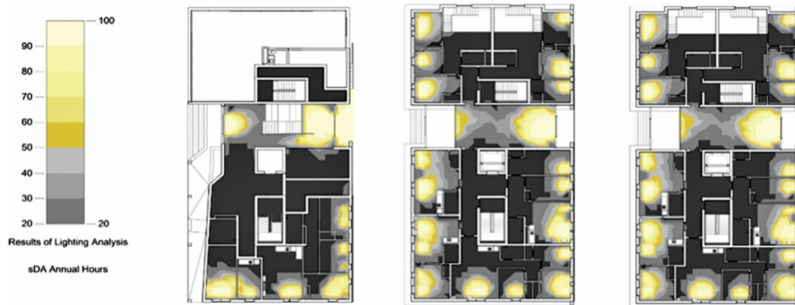
FIGURE 14: Spatial Daylight Autonomy Simulation. Spots in yellow comply with the daylight autonomy requirement of 300 lux for at least 50% of the year.
