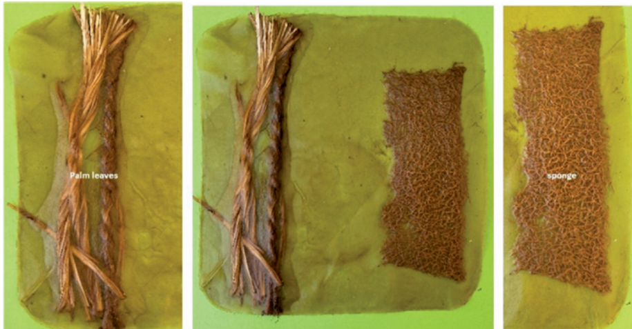
FIGURE 7. The BC + natural fibres film growth. By the authors.
