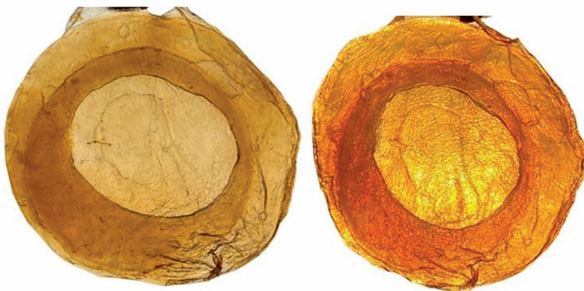
FIGURE 21. The resulting BC self-healed film after 7 days of fermentation, showing back and forth views, exhibiting material translucency and showing the welding edges between the two parts. By the authors.
