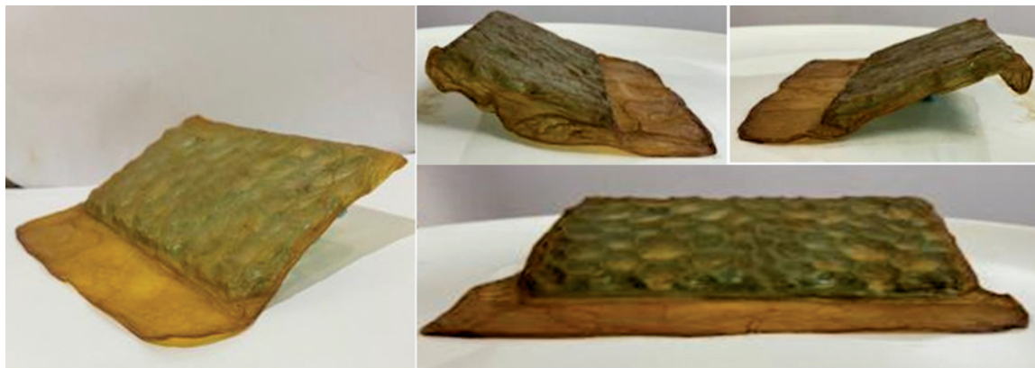
FIGURE 17. The dried BC film encompassing the 3D printed scaffold, after 3 days dehydration process. By the authors.
