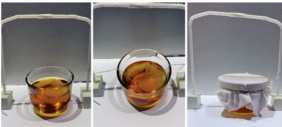
FIGURE 12. Inoculating the system with standard medium +the bioagent Acetobacter xylinum to produce the reinforced BC. By the authors.
