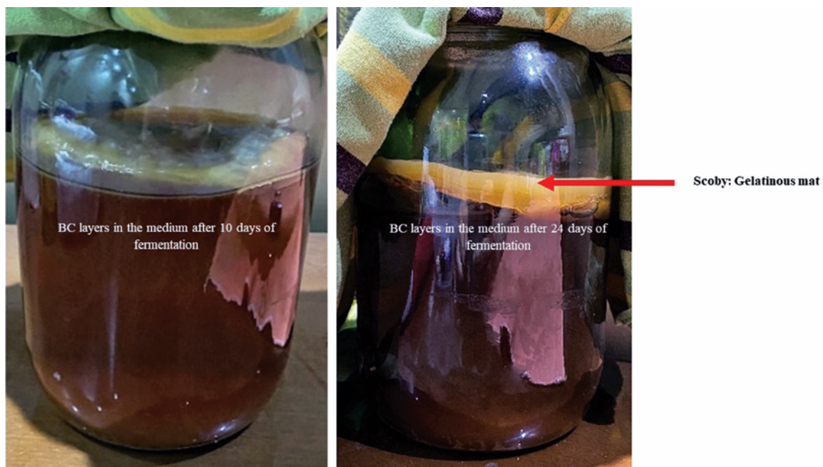
FIGURE 2. Different produced BC thicknesses, showing the relative growth in thickness of the Biopolymer film in relation to the incubation period. Left, BC formation after 10 days of incubation, Right, BC layers after 24 days of incubation. By the authors.
