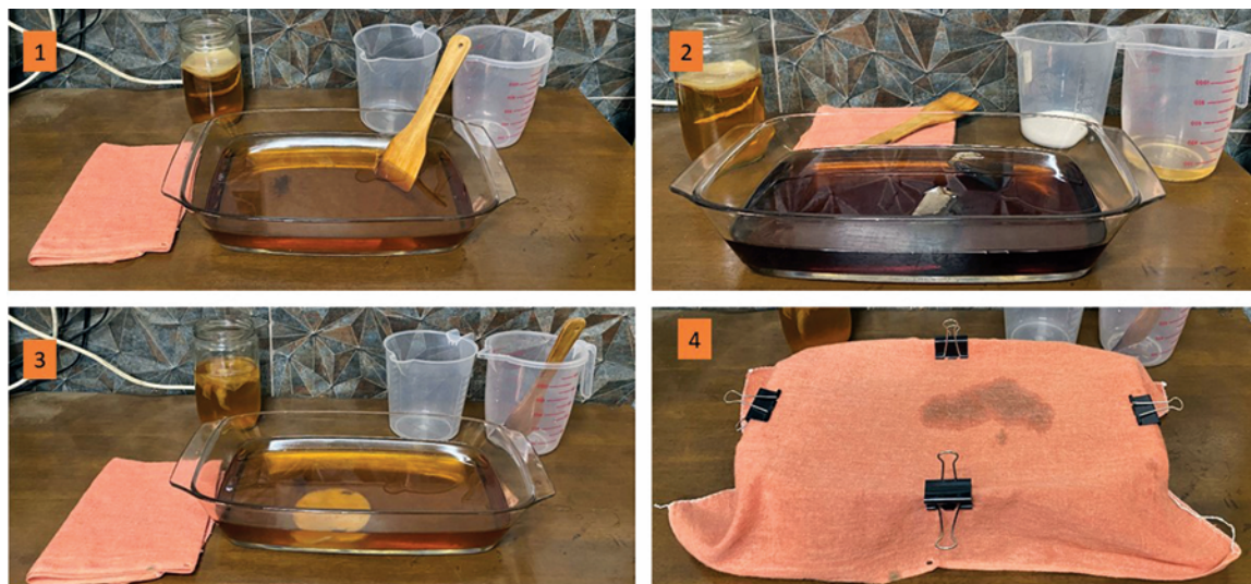
FIGURE 1. Bacterial cellulose simple production steps, that enables the autonomous mass production of BC on a personal scale, that will be utilized as an architectural material in different applications. Step 1: black tea bags were dissolved and stirred in 1000 ml boiling water and left to cool to 25°C. Step 2: 100 g of sucrose was added to the brew along with 100 ml apple cider vinegar. Step 3: the Scoby culture was added into the medium. Step 4: Finally, the container was covered with a light-blocking, air permeable cloth. By the authors.
