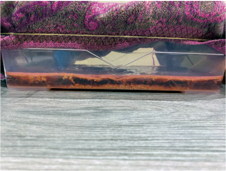
FIGURE 5. The produced BC after 8 days of fermentation, using organic waste as an alternative carbon source. The figure shows the pigmentation effect achieved by the organic waste of raspberry powder. By the authors.
