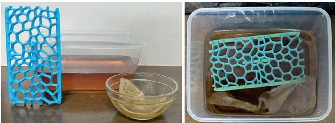
FIGURE 14. The preparation of the BC standard medium and the 3D printed scaffold, for customizing the formal properties of the BC film. By the authors.
