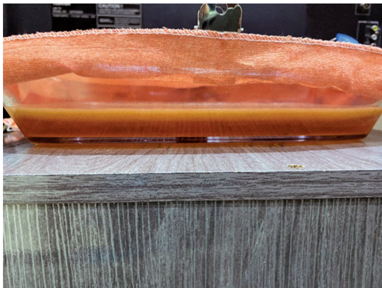
FIGURE 3. The resultant BC film after 10 days of fermentation using Acetobacter xylinum . By the authors.
