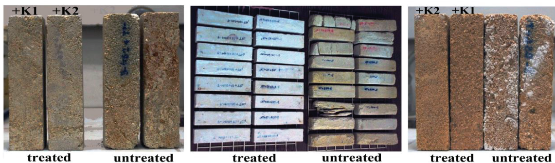
FIGURE 9. Treated and untreated new stones after salt crystallization test: (KS on the left; MS in the medium; BS on the right).
