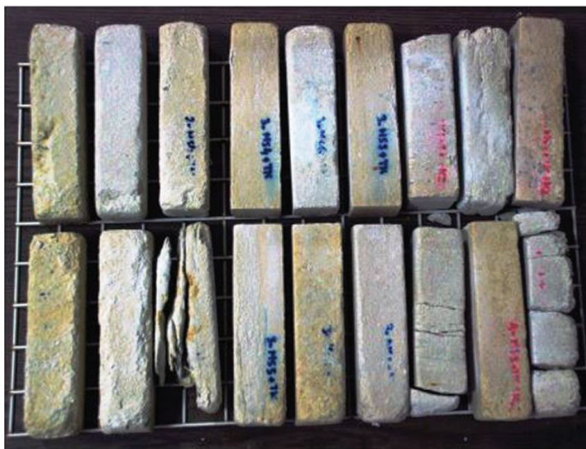
FIGURE 6. Meluša Stone after the 11th cycle of salt crystallization test.
