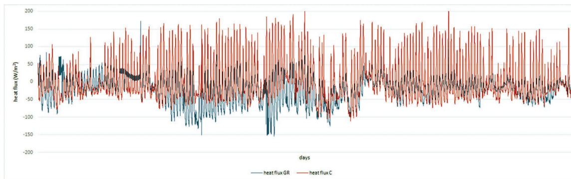
FIGURE 5. Heat flux patterns of green roof (GR in blue) and control roof (C in red) during the essay.
