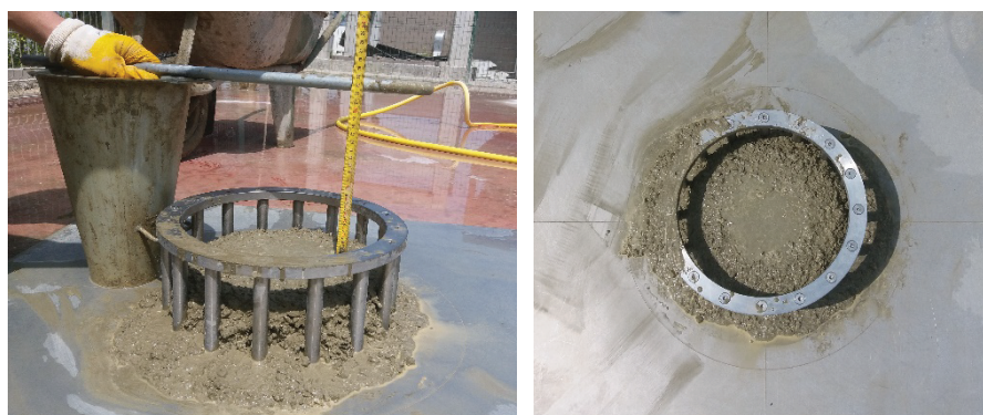
FIGURE 12. Blocking of SCC containing fiber between rebars of J-ring.
