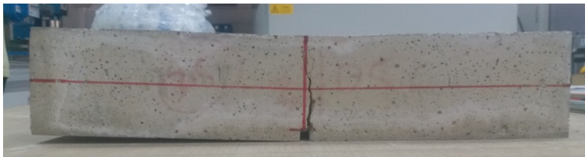
FIGURE 19. Crack opening after flexural test on fiber reinforced SCC.
