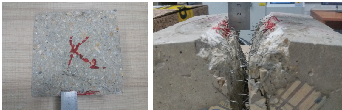
FIGURE 24. Measured of the depths of penetration of water; a. Control mixture; b. L30 mixture.
