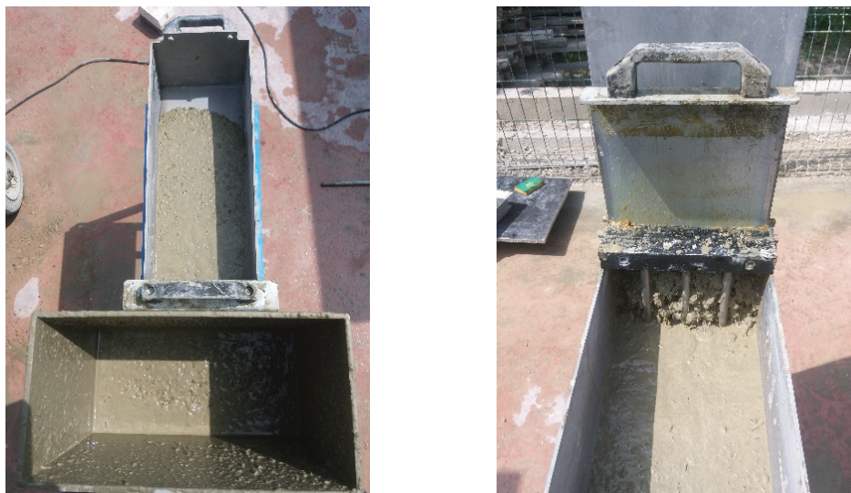
FIGURE 8. Blockage of SCC mixtures containing steel fibers in L-box.
