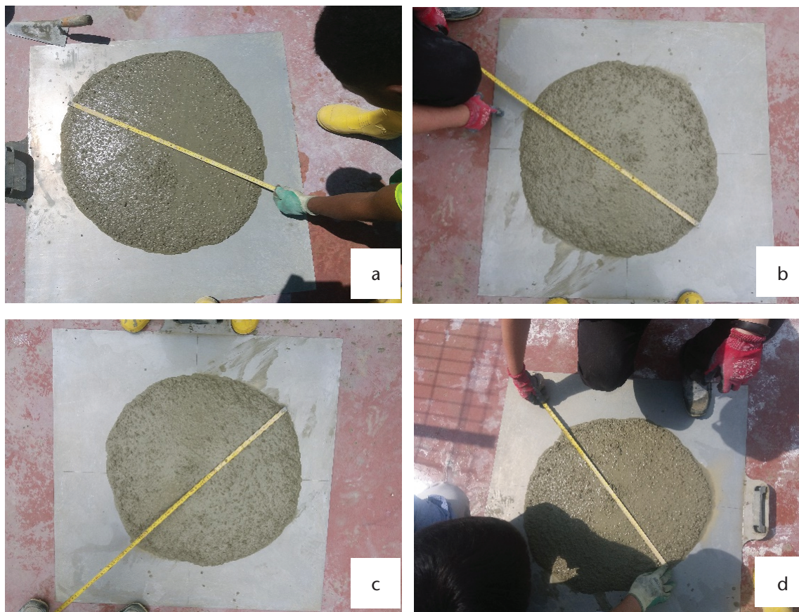
FIGURE 4. T50 slump-flow measurements of SCC mixtures; a. Control Mixture (C); b. L35 Mixture; c. L35 Mixture; d. L50 Mixture.
