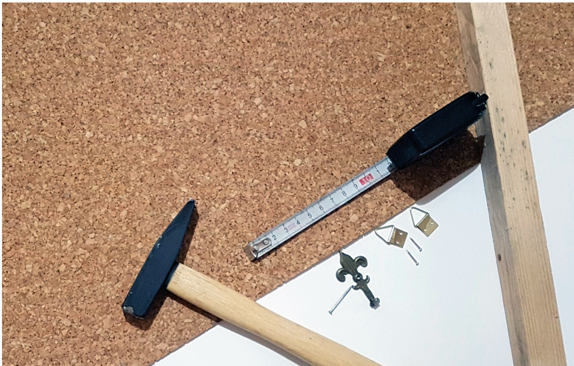
FIGURE 8. Details of the elements used to realize the sound-absorbing structure: hammer, tacks, hooks, wooden rod, and cork panels.
