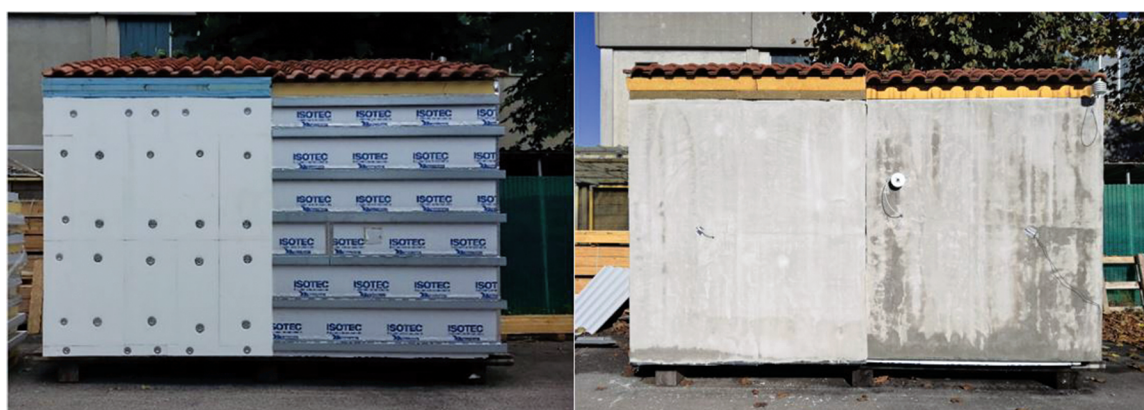
FIGURE 1. Test facility box installation phase of: (left) EPS insulation (West chamber) and micro-ventilated façade with Isotec® wall (East chamber); (right) finishing layers equal for both chambers.
