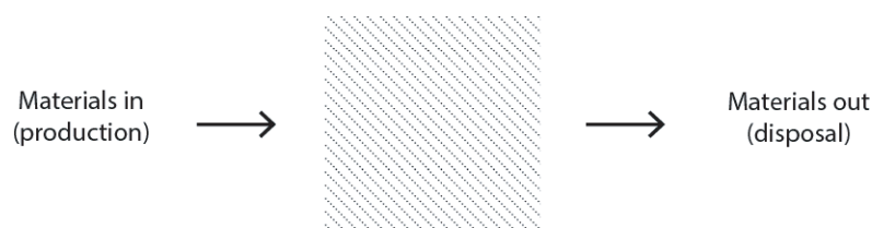
FIGURE 4. Refurbishment process ('black box' process). Environmental impacts are the sum of the new impacts added (through production of new products) to the building together with the impacts from the disposal (of the removed/replaced products). Thus, only obtaining insights into the overall processual behaviour considering only input-output, as the internal workings and mechanisms are not known.
