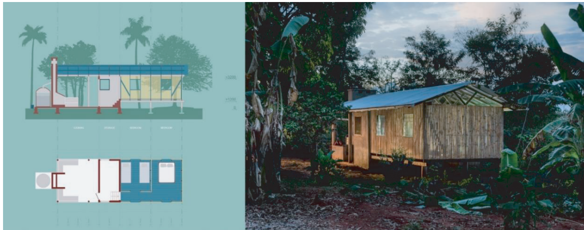
FIGURE 4. A prototype bamboo house designed by JBK (Ingvarsten Arkitekter, Copenhagen, Denmark) in the village of Magoda, in the Tanga region of Tanzania. Reprinted [adapted] from ArchDaily (2016).
