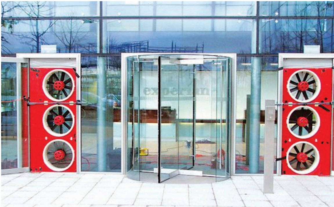
FIGURE 16. Blower Door Test in Commercial Building. Source: Urban Green Council Conquering the Energy Code presentation, 2017.
