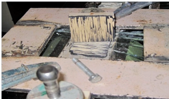
FIGURE 9. Cohesive failure in timber of a specimen tested in laboratory conditions.
