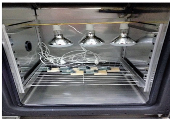
FIGURE 7. UV effect test in the climate chamber.
