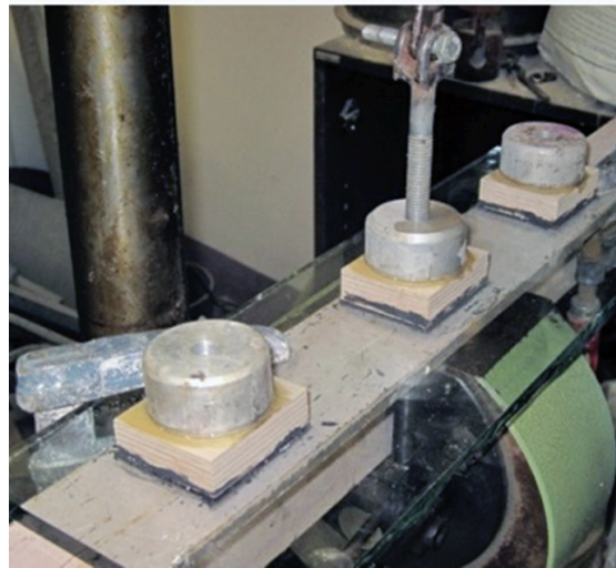
FIGURE 4. Test set-up of the uniaxial adhesion test.
