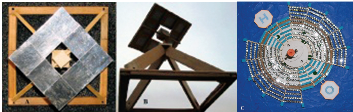
FIGURE 15. Supplemental case studies: A-B) small heliostats at peaks of skylight pyramid frames; C) hospital ship with small heliostats trusses on reused off-shore long wind blade beams and receiver tower above a storage (molten salt, firebricks) tank ballast model photo.
