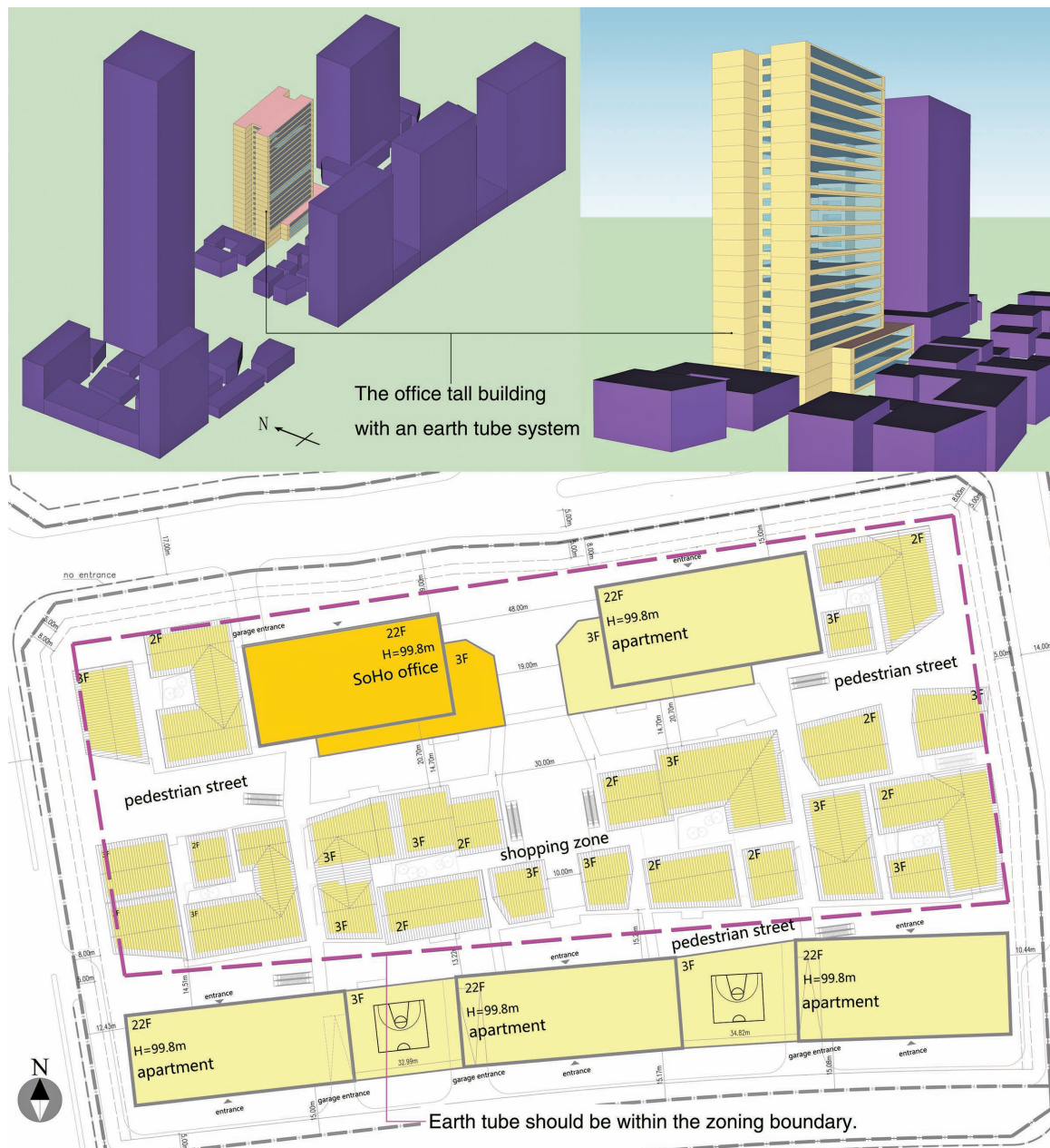
FIGURE 1. The mass model of the tall building and its surrounding buildings was established for energy simulation (Source: produced by the author); the site plan of the tall building (Source: Suzhou Wanyu Real Estate Development Co. Ltd.).
