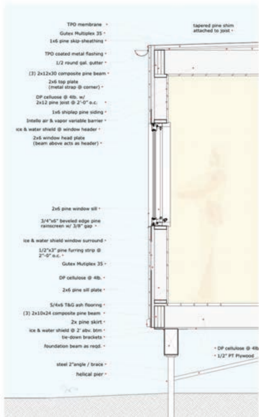
FIGURE 9. SUCASA Envelope Wall Section / image credit: Lutz
