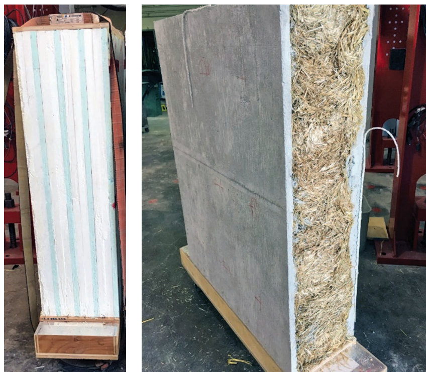
FIGURE 4. Tests specimens: characterization panels C1 (left) and plastered manufactured straw bale panel S5 (right).
