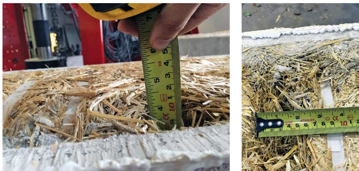
FIGURE 15. Example of voids in tested straw-bale panels: 40mm \times 100mm void through S5 (left) and 60mm \times 35mm void through S7 (right).
