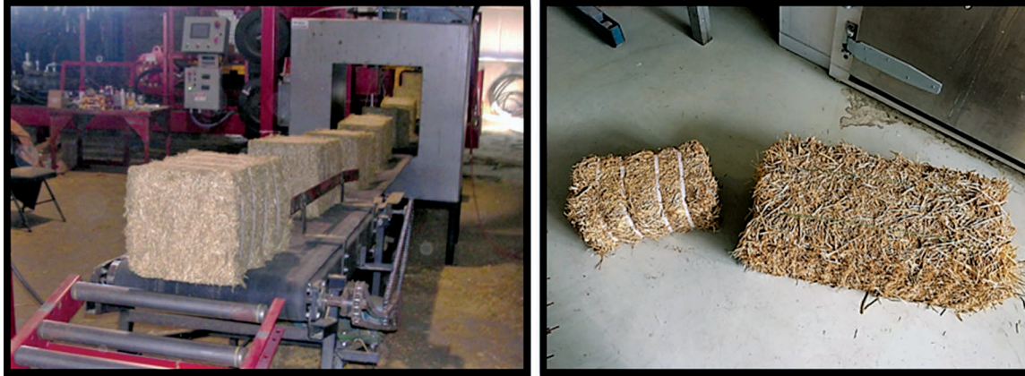
FIGURE 3. Manufactured baling process (left) and manufactured high density bale vs. regular 2-string bale (right) (Source: Olds Agtech Industries, 2008).
