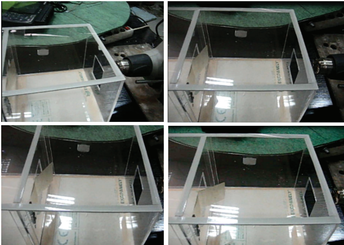
FIGURE 8. Shows the progress of the 2mm SMP sheet placed in the internal window within the model and exposed to hot air heated to 37 degrees Celsius, and it shows the movement of the sheet from 180 degrees to 45 degrees to 90 degrees, allowing the air to flow in the model.
